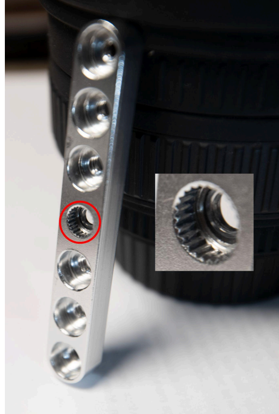
Functional arm with well defined splines
