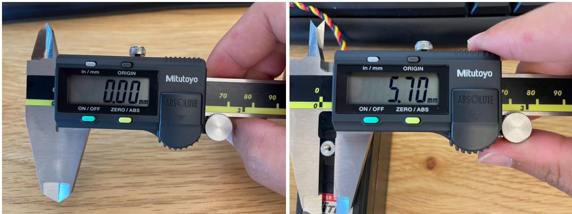
Ensure reading is 0 when fully closed
