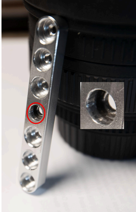
Worn out servo arm
